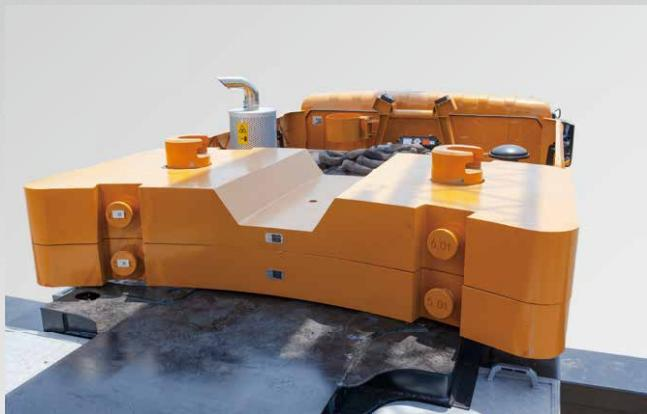
Fixed CW 3.7t, three movable blocks 5t, 6t, 6t, additional 2.5t\*2 for option. With CW base support available, the crane can travel with 20.7t CW on board at low speed in short distance.
