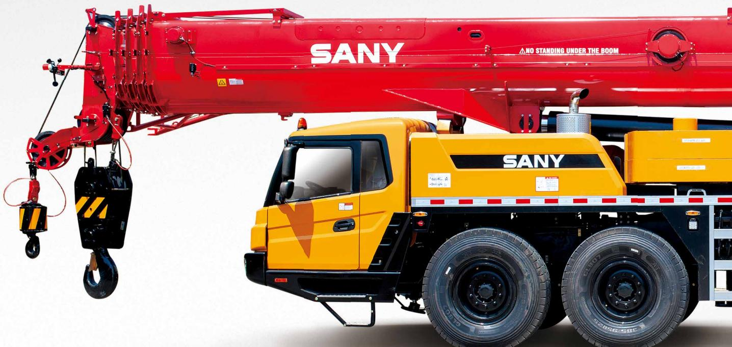
Remark :this illustration is crane with 20.7t counterweight for jobsite traveling.
