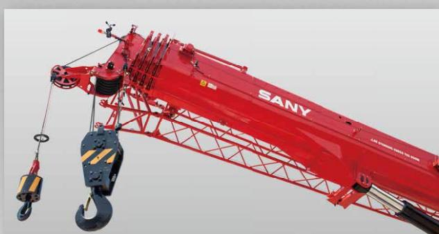
U shape large cross section 50m boom with 14.3t load capacity at full length, fixed jib 17.5m, 9.5m extension optional, leading in industry.
