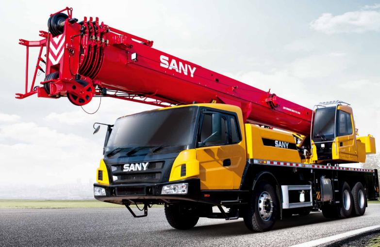
Max. Lifting Capacity: 30 t Max. Boom Length: 42.5 m
