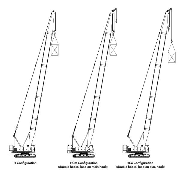
ConfigurationBoom ConbinationBoom LengthHBoomHCmBoom + Extension jib (double hooks, load on main hook)13m~52mHCaBoom + Extension jib (double hooks, load on aux. hook)
